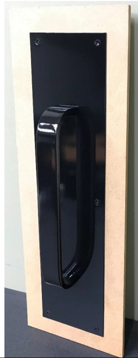
Aluminum Door Handle spray coated with AVM-S26
